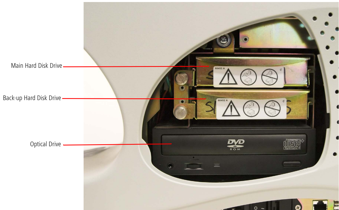
Figure 1-5 Drive Access Door Opened
