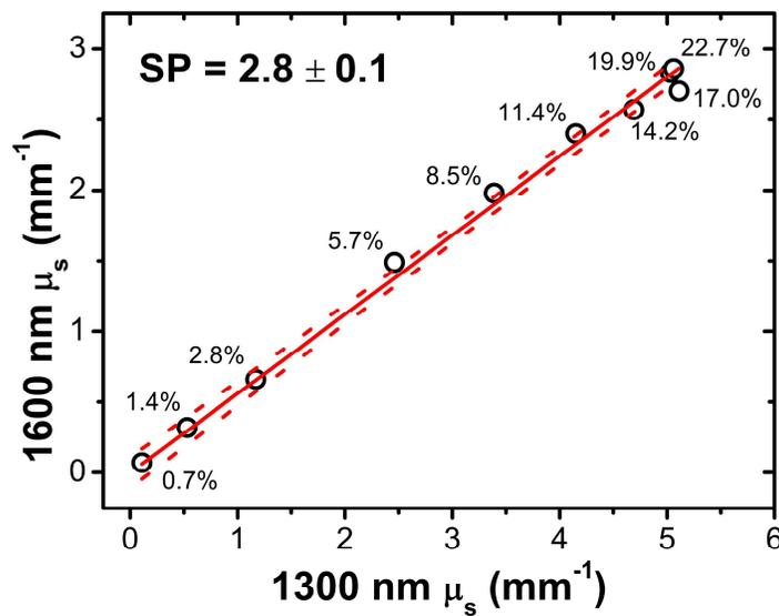
Fig. 5. Measured  $\mu_s$  at 1600 nm versus 1300 nm. Sample points are marked according to the Intralipid concentration. From a linear fit to the data (solid line) we determine the SP value for Intralipid (indicated). The dashed lines indicate the 95% confidence interval of the fit.
