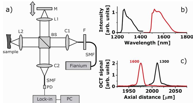
Fig. 1. (a) Overview of the time domain OCT set-up used in the experiments: BS – beamsplitter; C1,C2 – fiber collimating ports; L1, L2 – reference and sample arm lenses; M – reference mirror; SMF – single mode fibers; F – long pass filter; PD – photodetector; Lock-in – Lock-in amplifier; PC – personal computer; Fianium – supercontinuum light source; (b) OCT input spectra for the two wavelength bands; (c) coherence function at the two OCT wavelengths (measured with an OD3 filter in sample arm).
