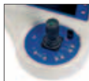
The Z-Ring accurately measures the position of each frame along the Z-axis thus enabling pachymetry
