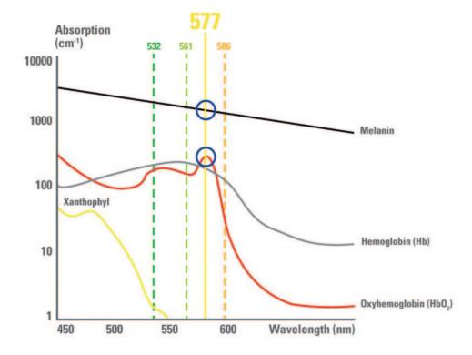
Compared to the commonly used 532nm green laser, the 577nm wavelength provides, better combined absorption by melanin and oxyhemoglobin, negligible xanthophyll absorption, low intraocular light scattering through partially-opacified media and high transmittance through cataracts.
