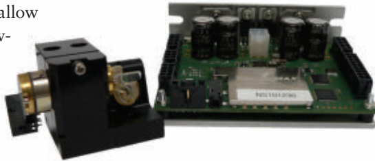
FIGURE 4. With speeds three times higher (and priced three times lower) than conventional galvo scanners, ScannerMAX requires less power, less physical space, and no external cooling.
