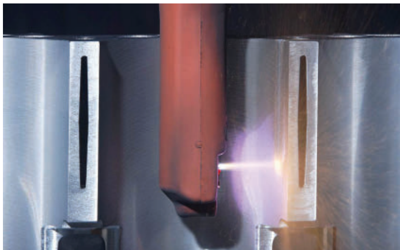
FIGURE 1. The cylindrical surface of a bore for an automobile engine is micromachined using a 2 kW single-mode fiber laser from IPG Photonics, then sprayed with plasma to create a hard coating that replaces conventional cylinder liners. Laser-machined microgrooves help the resulting coating to adhere to the cylinder. (Courtesy of IPG Photonics)
