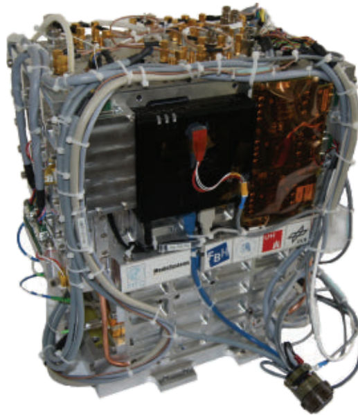
Thanks to careful engineering, the FOKUS optical frequency-comb module has been launched into space for a second time, performing without error and setting an important precedent for future research. (Courtesy of Menlo Systems)
