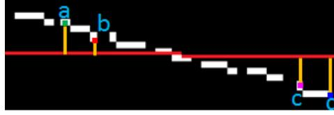
Figure 3.8: An example of the computation of the weight for finding the slope discontinuity ( $\psi$ ).
